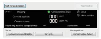
A test target can be changed in the "Select test target" screen by clicking the [Test Target Selection] button on the "Positioning test" screen.
